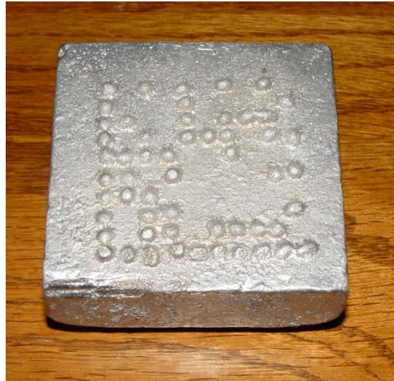
Figure 7: ISU group project cast symbol. Shown is a cast symbol that was readable.
