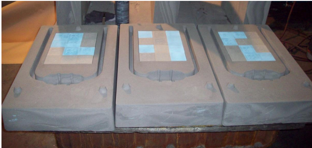
Figure 15: Experimental casting drag setup with symbol sand cores inserted into drag.
