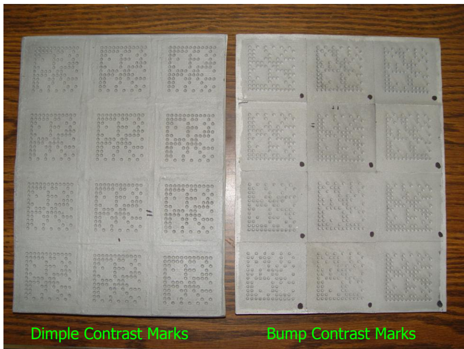
Figure 30: Cast specimens with Dimple and Bump mark geometry analyzed using DVT camera for Print Growth m and Symbol Contrast to further verify previous grading results.
