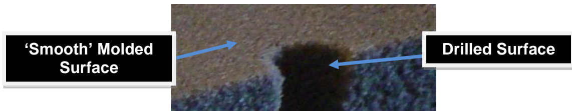
Figure 12: Cross sectional view of a drilled sand mark. The drilled surface is relatively rough compared to the molded core surface. Using pattern surface symbol geometry to create marks was used in as an experimental factor.
